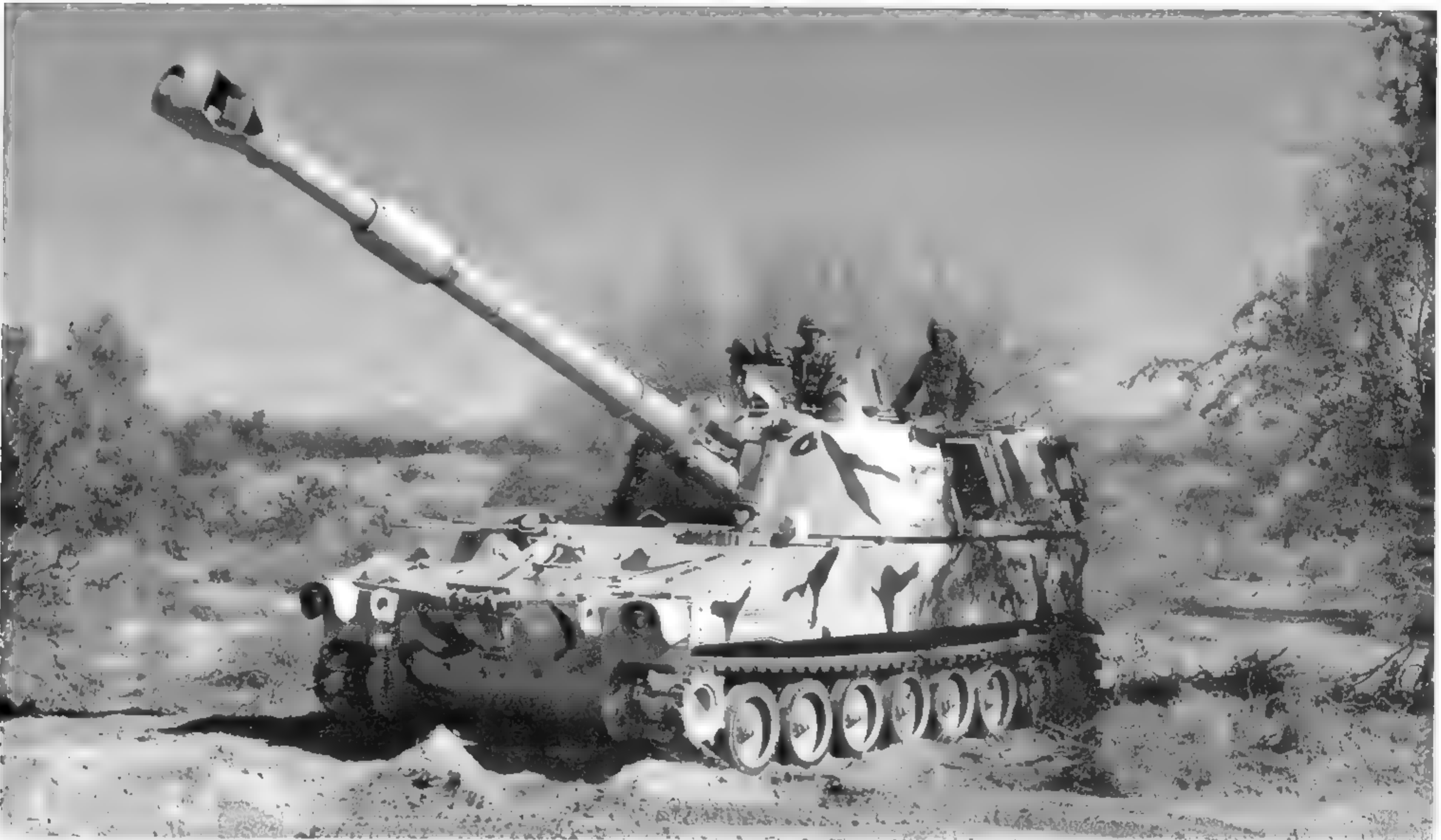
The M109A2 shown here lacked the flotation equipment of its predecessors, but featured an improved gun mount and an enlarged turret bustle. (Photo courtesy of United Defense)
